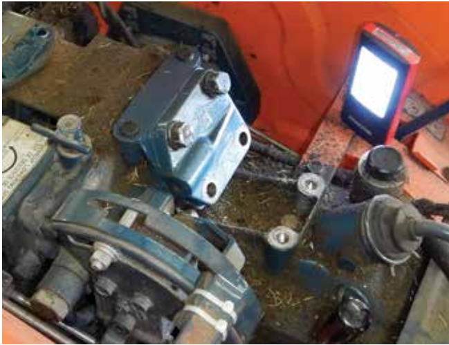
With the indexed bracket off, the head is exposed (clean the immediate area to reduce contaminants from entering cylinder before removing head)
