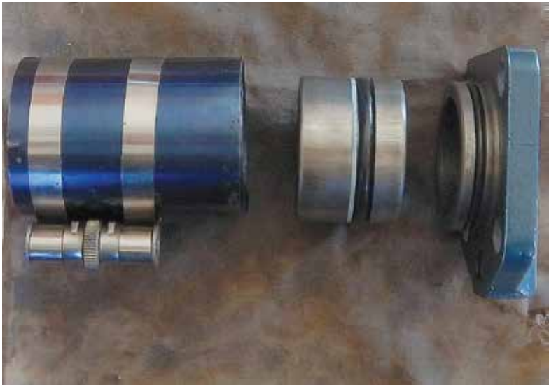
The piston ring compressor, piston and head with new rings
